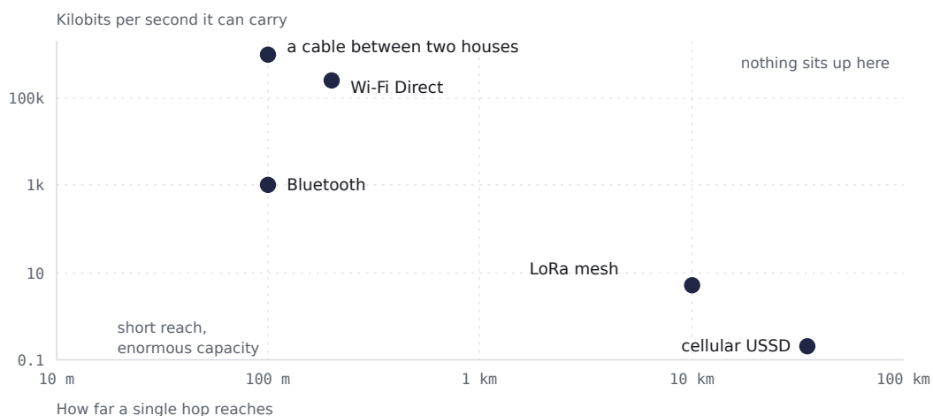
Figure 7: The top right of this chart is empty, which is why the design does not run agreement itself over radio. A LoRa hop cannot carry block traffic. It can easily carry a short signed line saying a provider has eggs today, and that is all the node needs to move.
